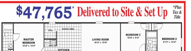
Price includes heat pump, 2 4x4 steps, plumbing, concrete footings, brick skirting, electrical hookup, setup, blocked & tied down & county permit.
