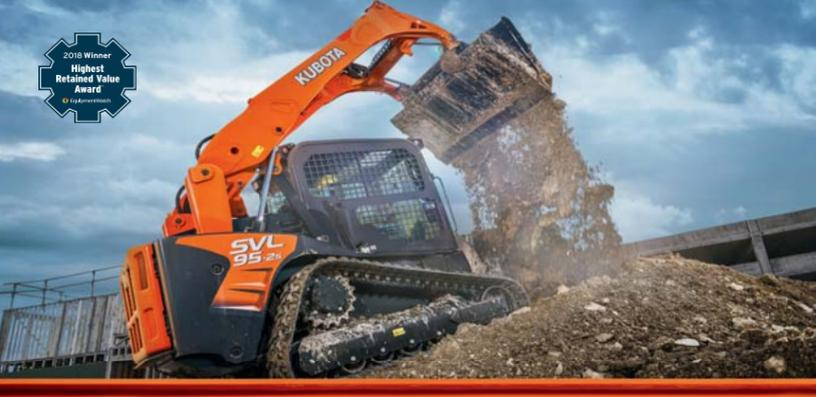
The proven 96.4 HP<sup>1</sup> Kubota engine powers the beast with 7,961 pounds of breakout force. A wider cab entrance, optimized AC and full-suspension seat provide all-day comfort. And an integrated mainframe and undercarriage handles any terrain, making the Kubota SVL95-2s seem almost unstoppable.
